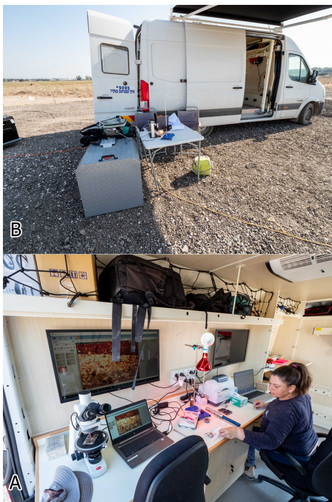
Fig. 2. View of the IAA mobile field laboratory in Yavneh during the excavation season of 2020. A) showing the interior of the lab with portable instrumentation such as microscopes and spectrometers. B) a general view of the vehicle, including instrumentation of a digital microscope and a fiber optic reflectance spectrometer (FORS).
